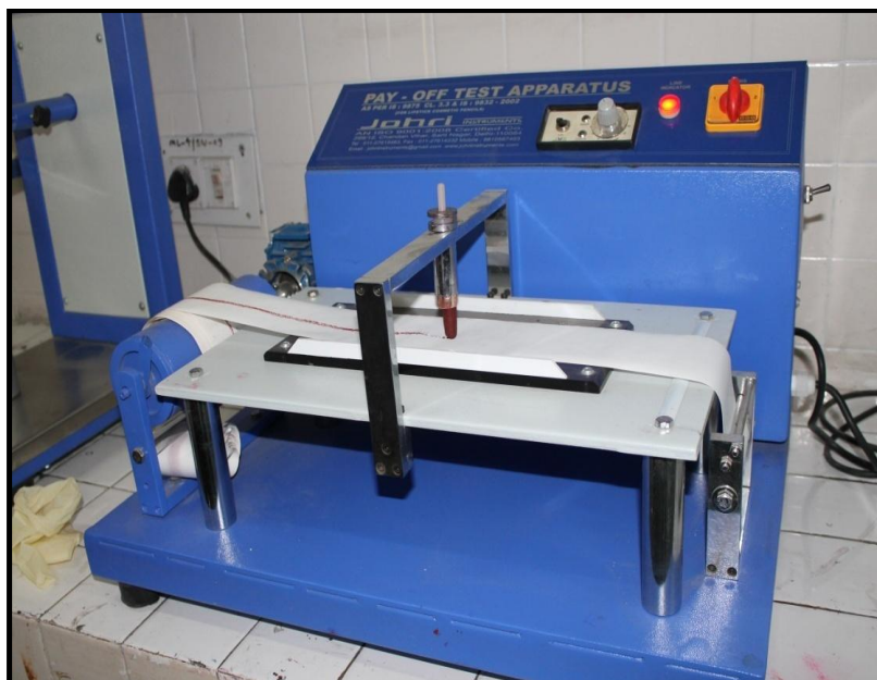
Figure-4: Pay-off test apparatus for lipstick salve
