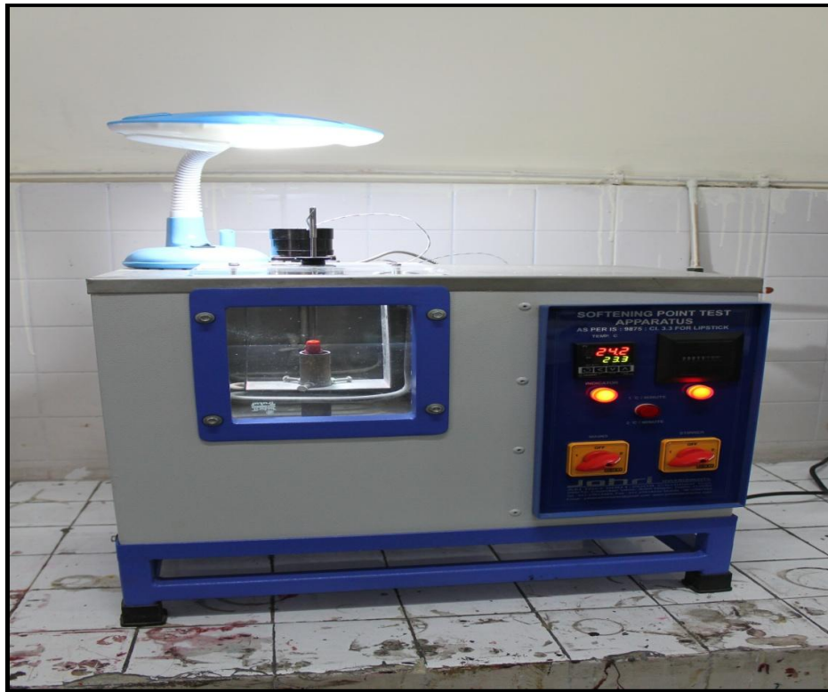
Figure-2: Softening point test apparatus for lipstick salve
