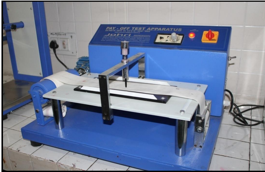
Figure 5: Pay-off test apparatus for cosmetic pencil
