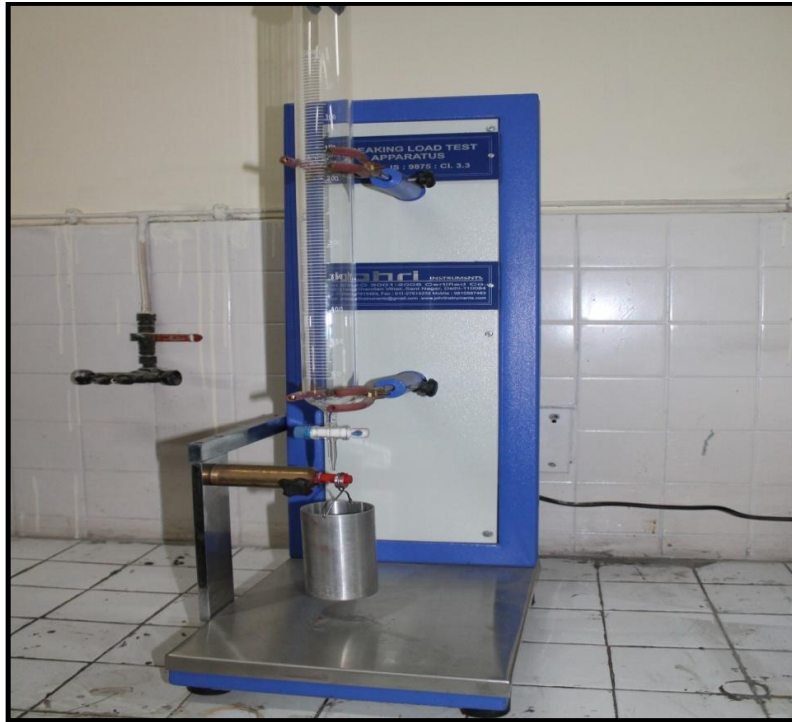
Figure-3: Breaking load test apparatus for lipstick salve
