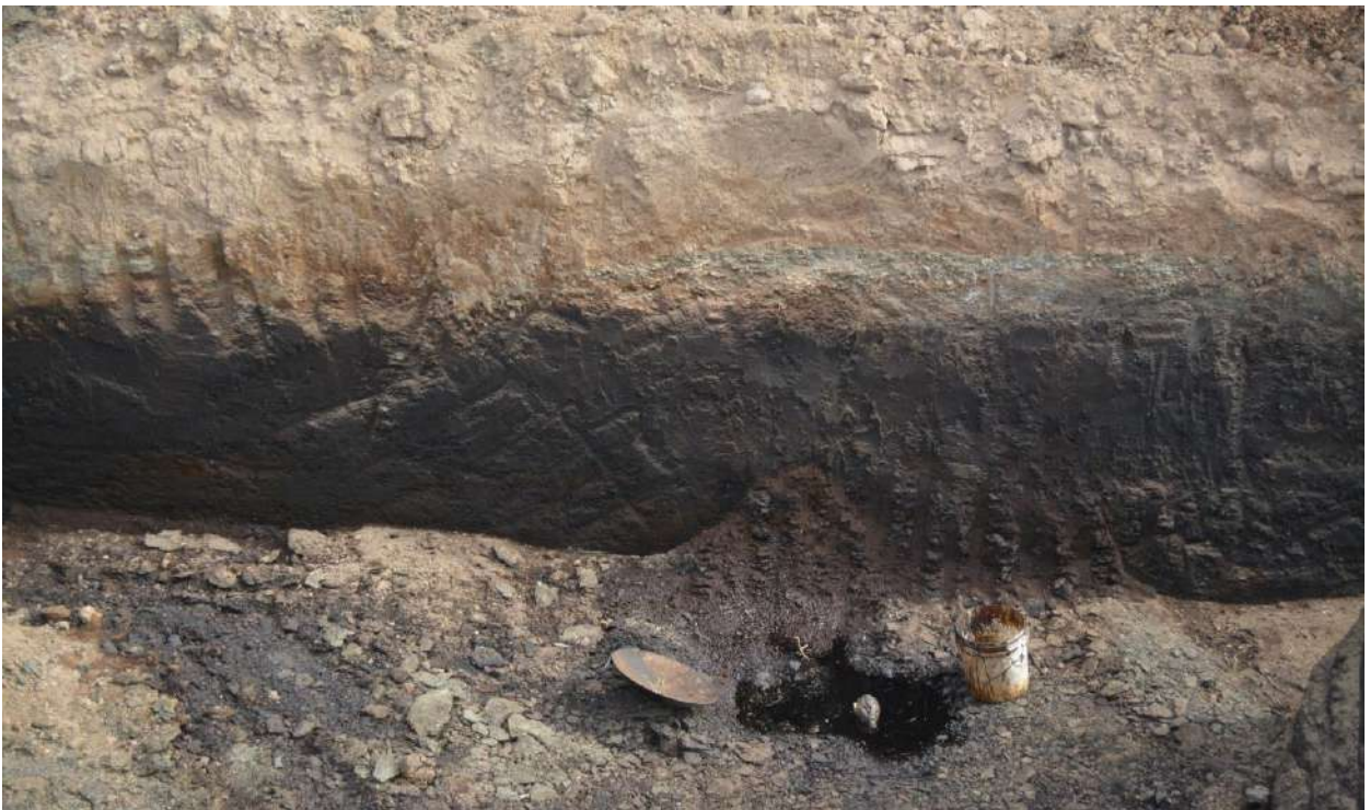
Figure 2: Vertical soil profile showing the sludge entrapped with spent wash in lagoon.
